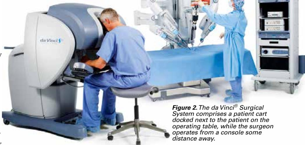
**Figure 2.** The da Vinci® Surgical System comprises a patient cart docked next to the patient on the operating table, while the surgeon operates from a console some distance away.
